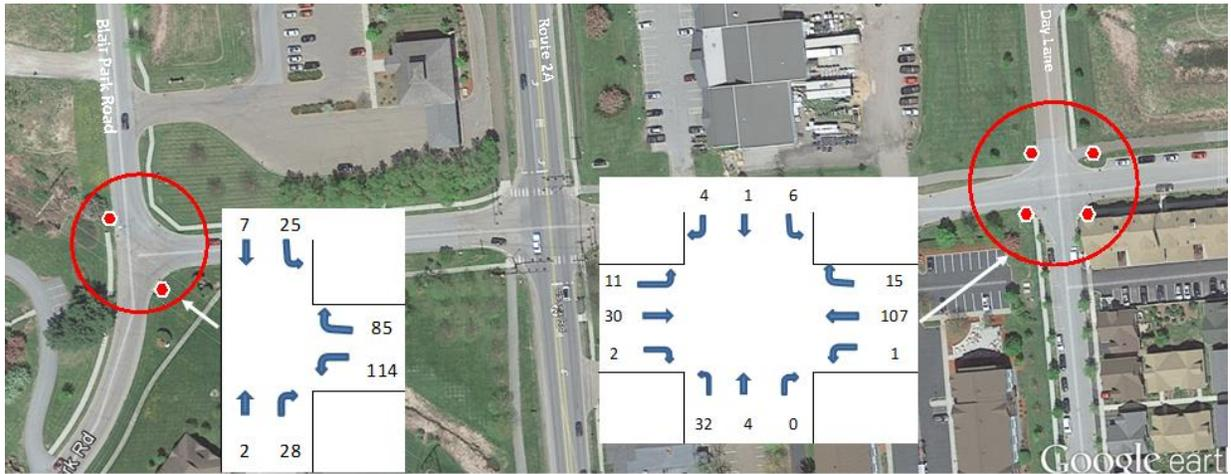
**Figure 3: PM Peak Hour Turning Movement Count**
