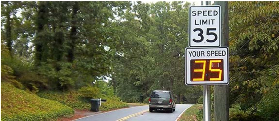
Sample of Speed Feedback Radar Sign
